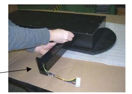
2. Have an assistant help you lift the header to the top of the game base with the printed areas facing forward. Make sure to feed the electrical connector into the hole on the top of the base cabinet.
