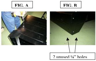
1. On a soft surface, lay the main machine on its front face (front has LED timer). With an assistant, position the base as so the flat front and back sections of the base are in the up and down position. Fasten the base to the machine by aligning the holes in the base with the holes in the bottom of the main machine and attach with (8) ¼ X 1" self threading screws (fig. C).
