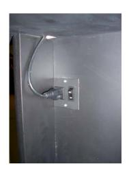
Plug the 3-way cord adapter into the outlet on the lid of the machine then plug the beacon and overhead light into the 3-way adapter.
