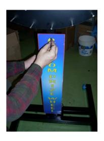
Install the wheel art plackard to the wheel. Make sure to line the six mounting holes on the plackard with the six screw inserts in the wheel before sliding the plackard over the pins. Secure the plackard to the wheel with (6) 10-32 X ½" (L) screws.
