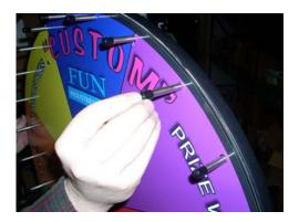
Install the clicker (I) to the clicker shaft above the wheel with (1) 10-32 X 1" hex head screw (J). Insert the screw from the right side and tighten securely.
