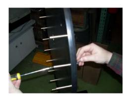
Install the header to the front of the main pole above the wheel with (2) 10-32 X 1" (N) screws.
