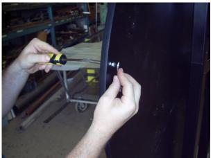
21. Attach the printed plastic header and wheel panels to the header and wheel with (8) 10-32 x  $\frac{1}{2}$ " screws. Align the holes in the wheel panel with the six screw inserts in the wheel before sliding the panel over the wheel pins.
