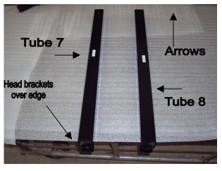
12. Locate and attach upper mast brace (MB3) using (4)  $\frac{1}{4}$ -20 x  $\frac{1}{2}$ " screws to the inside of tubes 7 & 8. Make sure the decal is face up and the arrows on the brace are pointing the same direction as the arrows on tubes 7 & 8. The clicker shaft will be pointing downward and it will make attaching this part easier to allow the shaft to hang over the assembly bench as well. Do not fully tighten.
