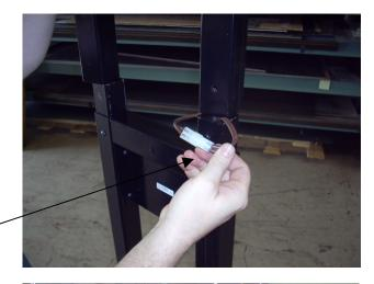
14. Once the rope light cord has been connected and tucked into the tube, slide the upper mast down onto the lower mast splice tubes and attach with (2)  $\frac{1}{4}$ -20 x  $\frac{1}{2}$ "screws. You may have to loosen the screws in the lower mast for alignment. Make sure the clicker shaft at the top is pointing forward (away from you) as well as the wheel shaft. You may now fully tighten all upper mast screws.
