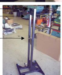
16. Locate and attach the wood header to the brackets at the top of the upper mast with (2) 10-32 x 1" screws. This step may require use of a step ladder. Use the two thru holes toward the center of the header. Make sure the rope light is facing forward and the cord does not get pinched on the back side. Fully tighten.
