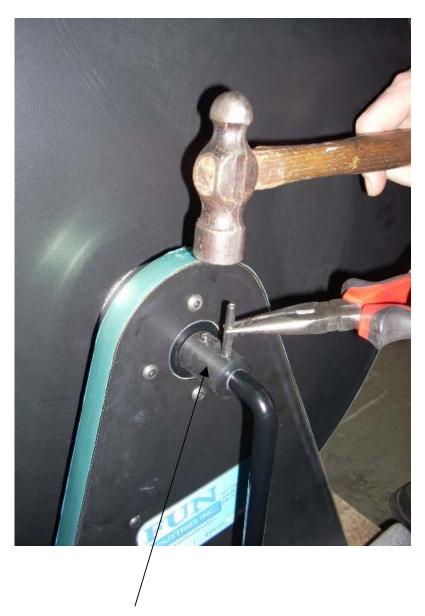
ATTACH CRANK HANDLE TO COUPLER WITH ROLL PIN
