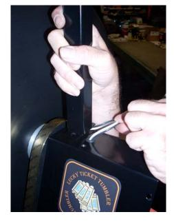
8. Attach the sign box assembly to the tumbler motor box and idle end bracket with 4 screws.
