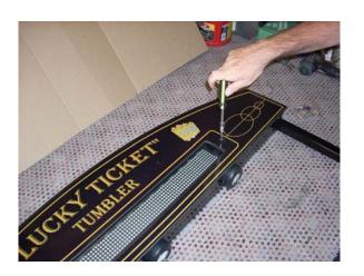
6. Attach the sign box assembly to the tumbler. Start by removing the 5 screws on the motor side cover. Remove the side cover and set it aside.
