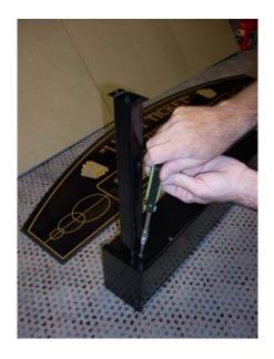
5. Attach the graphics panel to the front of the message sign box with 2 screws. Fully tighten.
