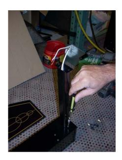
4. Attach the remaining support tube to the other end of the sign box with 2 screws. Fully tighten.
